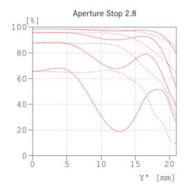
The MTF is indicated both at full aperture and at f/5.6 at long taking distances (infinity). Shown is the contrast in percentage for 5, 10, 20 and 40 lp/mm accross the height of the 35 mm film format, for tangential (dotted line) and sagittal (solid line) structures, in white light. The 5 and 10 lp/mm will give an indication regarding the contrast ratio for large object structures. The 20 and 40 lp/mm records the resolution of finer and finest object structures.
