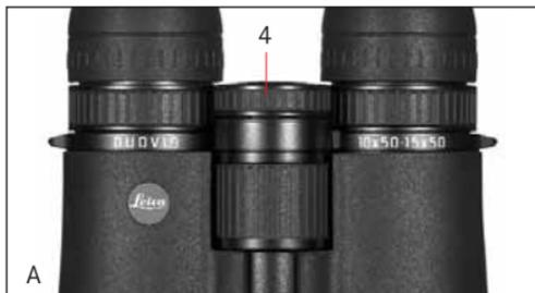
Compensation for individual defective vision for viewing without eyeglasses is made using the diopter ring (4), which is normally locked. (Figure A). First of all, the central focusing ring is used to focus the *right* barrel on an object. The diopter ring is then released by pulling it up. (Figure B).
